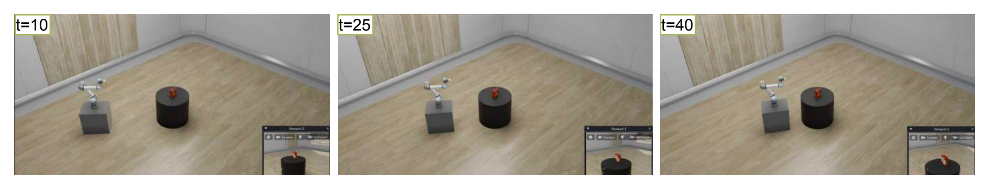
Policy learnt by the robot to approach the object it intends to grasp by respecting the vision constraints (keeping object in the center of image to allow better object pose tracking) using its base and arm wrist joint motion.
