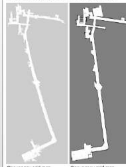
Comparison between occupancy grid maps created using SLAM and OSM based approach. Both maps look similar.
